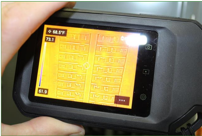
6.12 Item 1(Picture) Testing for Hot Spots
