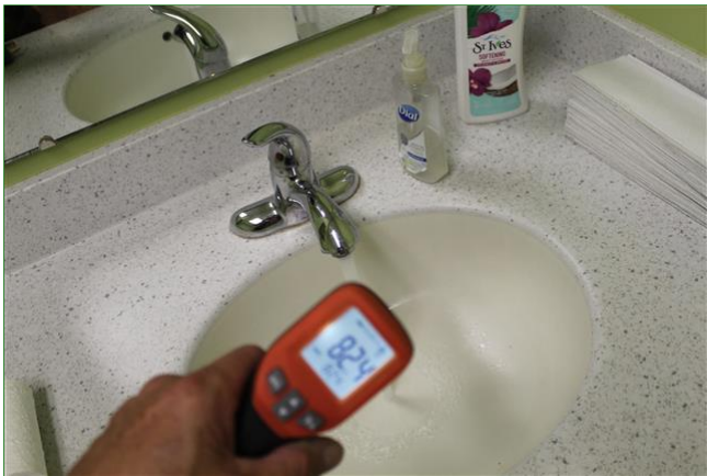
5.8 Item 3(Picture) Water Temperature Testing
