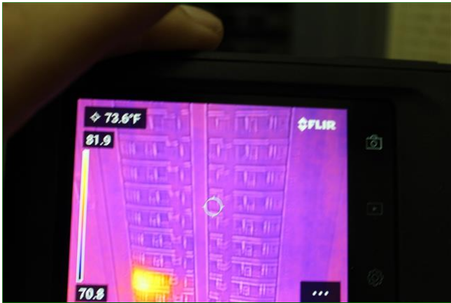
6.12 Item 6(Picture) Testing for Hot Spots
