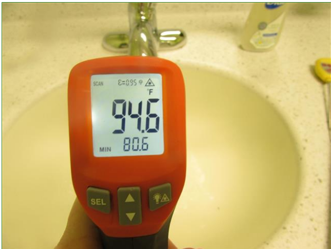
5.8 Item 7(Picture) Water Temperature Testing
