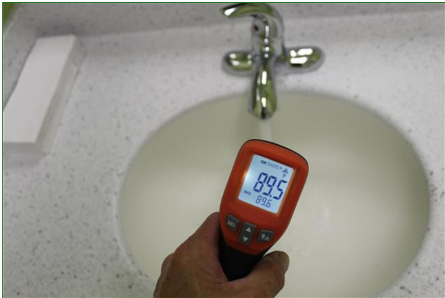
5.8 Item 1(Picture) Water Temperature Testing
