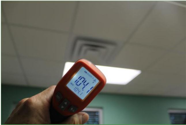
4.6 Item 6(Picture) Testing - Heating Mode
